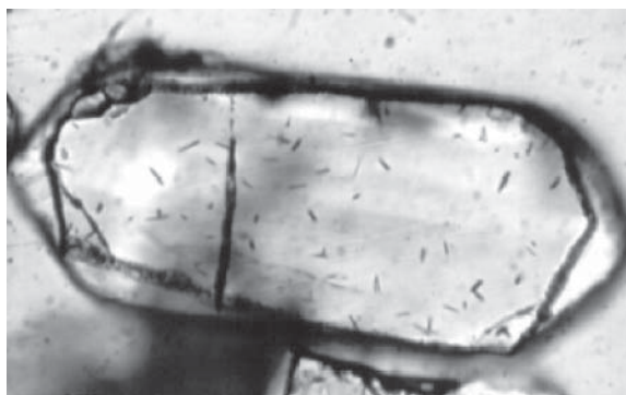
Figure 4.14 Fission tracks in a polished and etched zircon. (Source: Photo by J. M. Bird. Reproduced with permission.)
