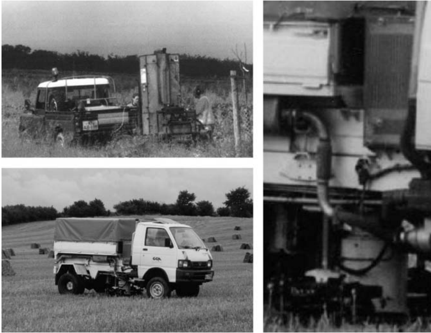
Fig. 2.5. Examples for seismic sources applied in near surface prospecting: Accelerated weight drop (THOR Geophysical, Kiel) (top left) and small Vibroseis ® truck (GGA-Institut, Hannover) (bottom left). The piston and ground plate through which hydraulic movement of the Vibro-truck is transferred to the ground are shown on the right hand side
