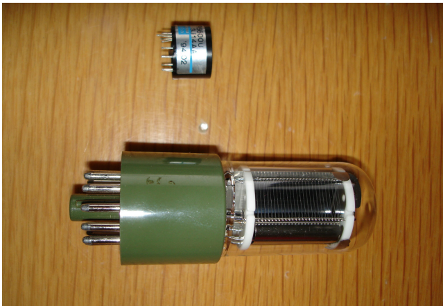
Fig. 3. Side-window PMT (bottom) and compact size PMT (top).
