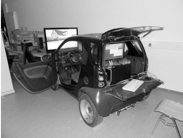
Fig. 2 Virtual Test Drive driving simulator with a complete vehicle mock-up
