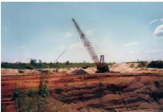
Fig. 96 Drag-line set-up of diamond bearing gravels in Banankaro in the Kerouane region.
