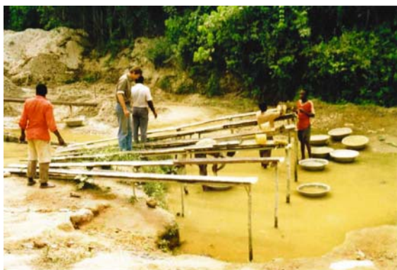
Fig. 92 Chutes for liquid clayey gold mud used in artisanal mining in the Ashanti region
