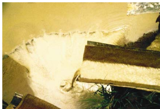
Fig. 93 The siphon of a liquid gold mud delivering chute in the Ashanti region
