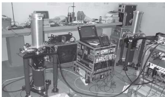
Fig. 7 Parallel measurements with FG5-220 (IfE) and FG5-221 (FGI) at station Metsähovi in Finland.
