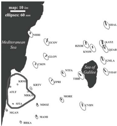
Fig 4. The error ellipses of the points, according to the Carmel datum, that bound with the thick closed line, \alpha = 0.05 . The lines start in the ellipses center sign the displacements.
