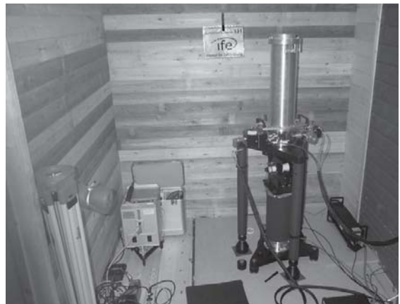
Fig. 6 Absolute gravimeter FG5-220 of IfE installed at station Östersund.
