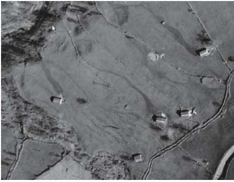
Fig. 6. Infrared aerial image. It is possible to observe the domestic wastewater discharges emitted into the environment from the rural houses.
