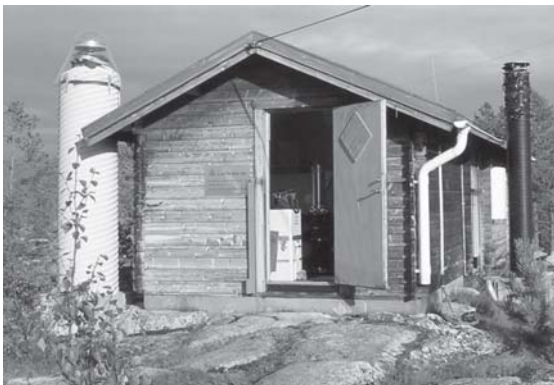
Fig. 5 Station Skellefteå (Sweden) with an absolute gravity pier inside and permanent GPS antenna outside.
