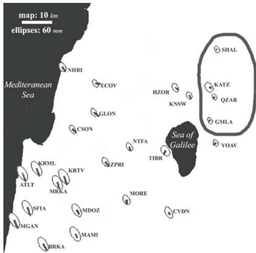
Fig 6. The error ellipses of the points, according to the Golan Heights datum, that bound with the thick closed line, \alpha = 0.05 . The lines start in the ellipses center sign the displacements.
