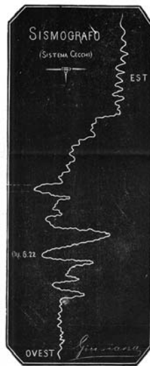
Fig. 28.5 Seismogram of the Ligurian earthquake of 23 February 1887, recorded at the Moncalieri Observatory with the UCEA’s restored Cecchi electrical seismograph with sliding smoked paper. The recording, published in Denza (1887) regards the EW component, while Denza himself states that the recordings of the remaining 3 components (NS, Z and “whirling movements”) did not present significant traces
