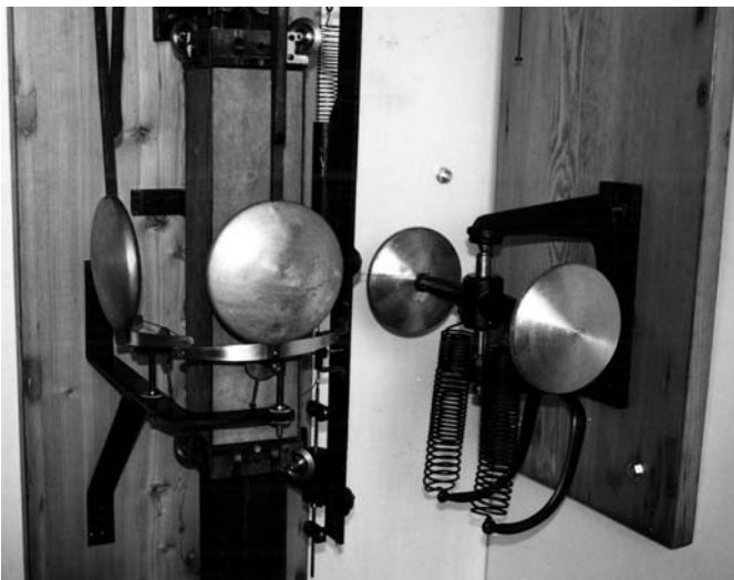
Fig. 28.4 Particular of the Cecchi electrical seismograph with sliding smoked paper (Cecchi 1875) showing the recording system (on the left) and the apparatus for the surveying of the so-called “rotational” movements
