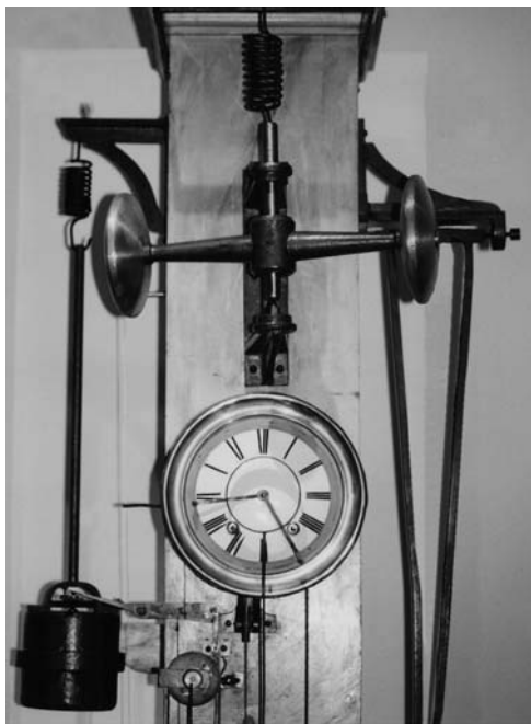
Fig. 28.6 The Cecchi electrical seismograph with sliding smoked paper – second model (1880s), particular of the detection system of the so-called “rotational” movements
