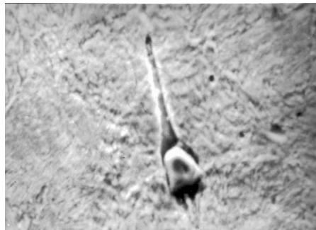
Figure 2. Rest of a lead particle in a steel barrier, \times 5,000
