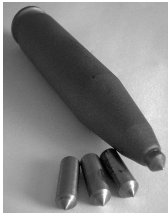
Figure 13. Self-sharpened mining tool and metal blocks from the composite tool material
