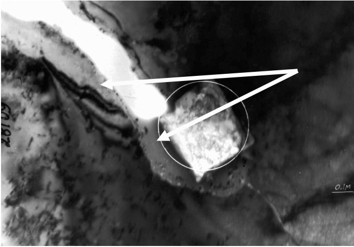
Figure 7. Zone of braking of Si striker of the cubic form, \times 60,000
