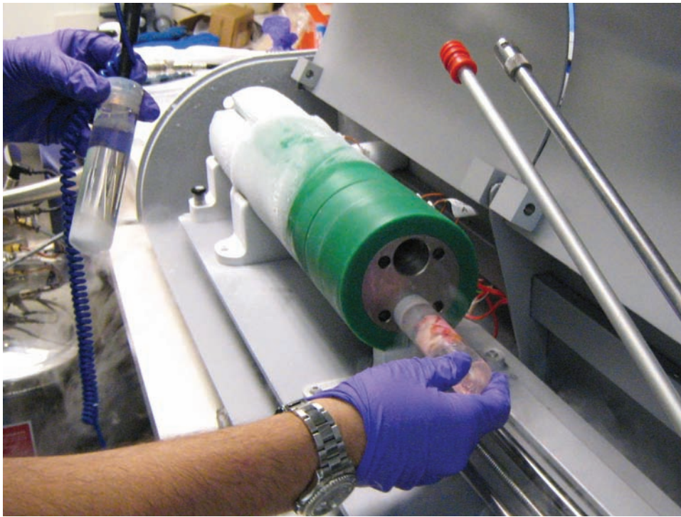
Figure 30.2 Whole human ovary cryopreservation with the vascular pedicle utilizing the same Multi-Thermal-Gradient device and slow cooling, rapid thawing protocol as described in the text.
