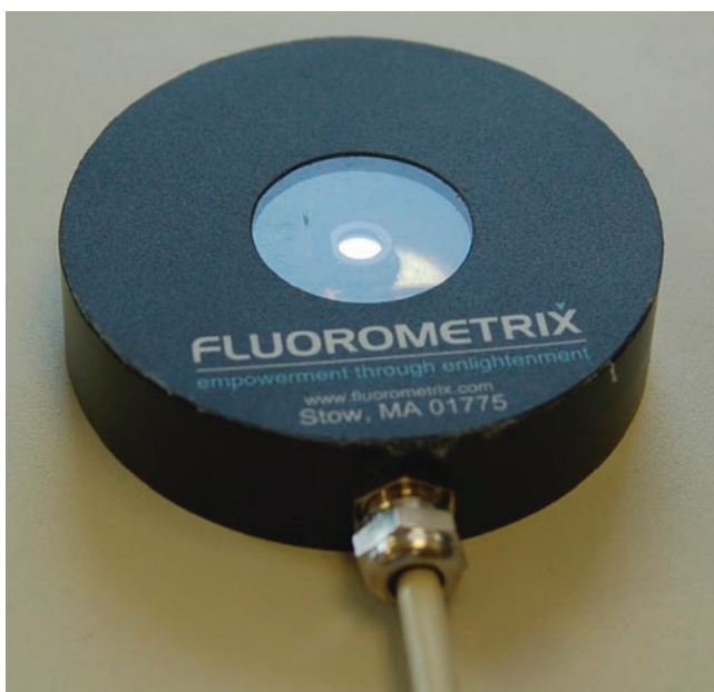
Fig. 10 An optical DO sensor based on phase shift measurement
