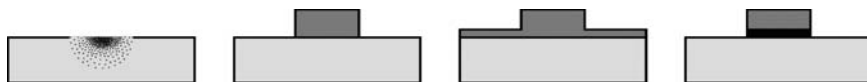
Fig. 6 Different types of channel waveguides – from left to right, ion-exchange, channel, ribbed, ARROW
