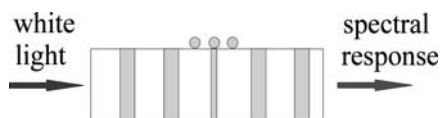
Fig. 8 Experimental scheme of a spectral transmission experiment of a photonic crystal Bragg reflector micro-cavity fabricated out of refilled holes in silicon. The central refilled hole acts on a nanocavity. AuNPs are immobilized in and around the central nanocavity
