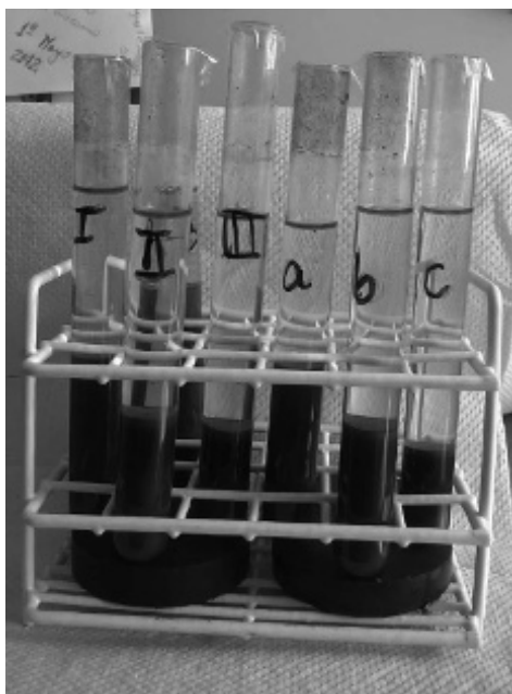
Figure 7.12 Demulsification after 6 months (magnetically assisted).
