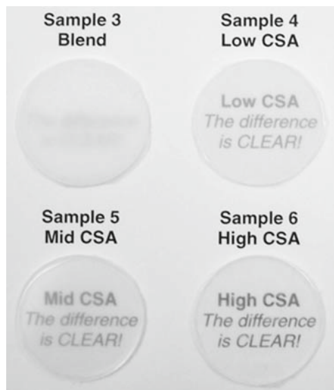
Fig. 18 Several samples of ethylene-octene copolymers having similar comonomer content, crystallinity, and melt index. Sample 3 is a physical blend of high and low density copolymers. Samples 4–6 are OBCs prepared with several different levels of chain shuttling agent. Reproduced by permission from [10]
