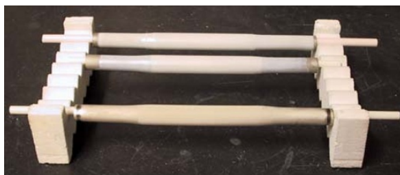
Fig. 12.4 Two Pall AccuSep \text{ZrO}_2 coated porous stainless steel filters at top. Pd coated AccuSep filter at bottom. These substrates have approximately 30 \text{cm}^2 of active area
