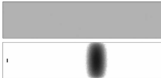
Figure 1. Solute transport in a homogeneous medium. Top Hydraulic conductivity distribution. Bottom “Snapshot” of a solute plume being transported through the homogeneous medium (the black rectangle on the left denotes the initial solute distribution). Spreading and mixing processes are due to local dispersion
