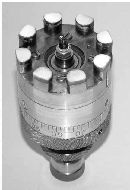
Fig. 2.4. A polishing jig that allows for adjustment of the tilt angle in an arbitrary azimuthal direction (courtesy of Udo Linke). A bead crystal is mounted for illustrative purposes. The bead crystal is embedded into meta-acrylate before polishing.
