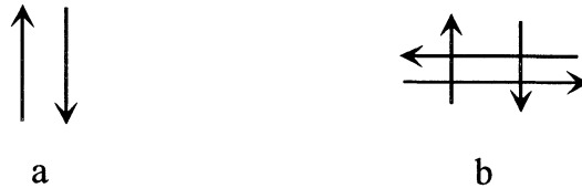
Figure 7.6. Schemes of acting forces in the earthquake hypocenter: (a) dipole, (b) double force couple.
