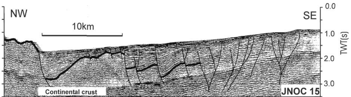
Fig. 5.4-3. Multichannel seismic profile JNOC15 showing the main structures across the western Bransfield Basin
