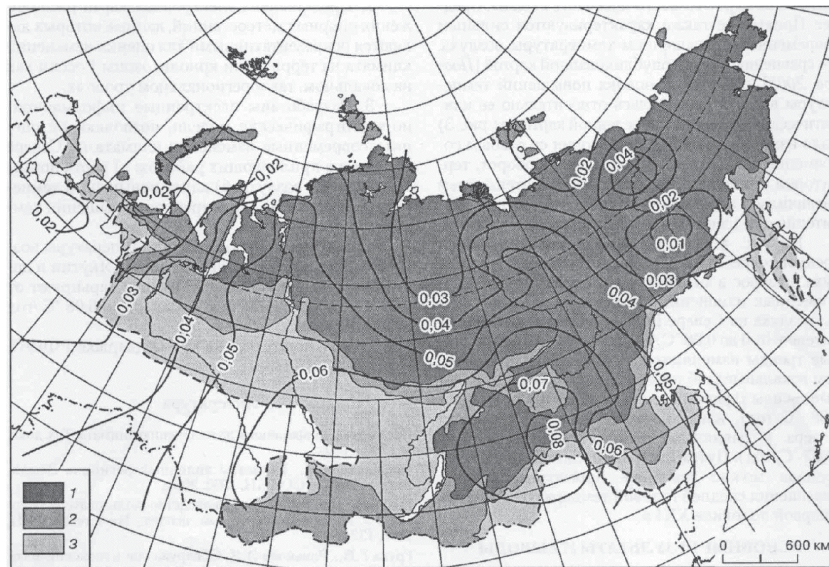
Figure 3. Map of increasing T_s trends (°C/year) derived from observations at meteorological stations in 1960-2000 (Pavlov and Anan'eva, 2004). Types of permafrost: 1 - continuous, 2 - faltering, 3 - island.
