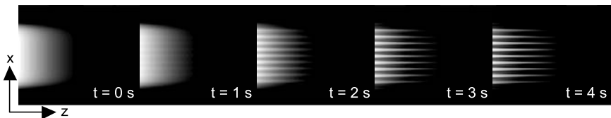
FIGURE 9.17. Numerical simulation of the model equations 15–17 ( A_2 component is depicted). The mirror is to the right of each time frame, such that the beam propagates to the left.
