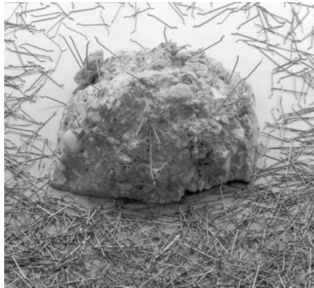
Fig. 5.7. Steel fibres and steel fibre reinforced shotcrete 5
