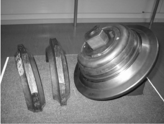
Fig. 4.65. Disc cutters from Lötschberg base tunnel. Left: Worn disc cutters
