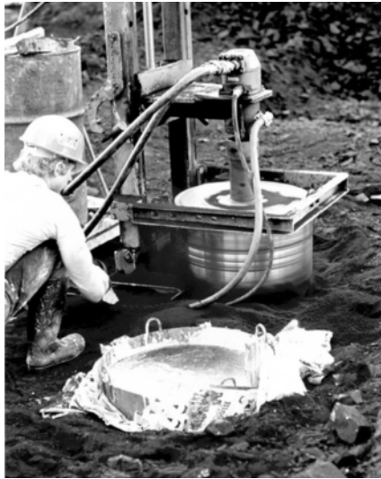
Fig. 3.3. Drilling of large core sample ( \varnothing 60 cm)
