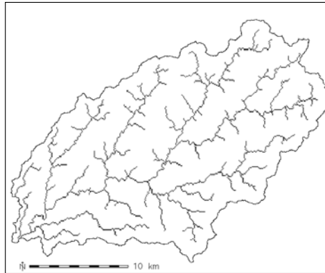
Figure 4b. Stream network derived using r.watershed and 100-m grid cells.
