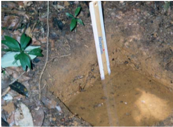
Figure 6. Measurement of upper limit of infiltration rates in small test pits.
