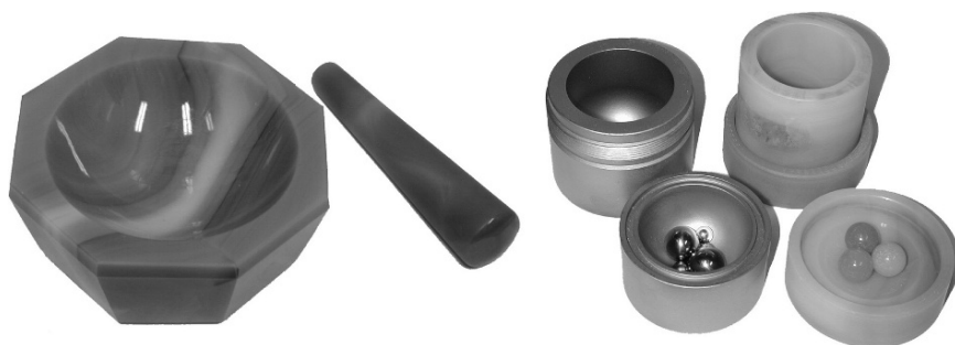
Fig. 12.2 The tools most commonly used in sample preparation for powder diffraction experiments: agate mortar and pestle ( left ), and ball-mill vials made from hardened steel ( middle ) and agate ( right ).
