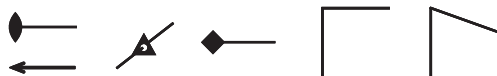
Fig. 2.4 From left to right : horizontal twofold rotation axis ( top ) and its alternative symbol ( bottom ), diagonal threefold inversion axis inclined to the plane of the projection, horizontal fourfold rotation axis, horizontal, and diagonal mirror planes. Horizontal or vertical lines are commonly used to indicate axes located in the plane of the projection, and diagonal lines are used to indicate axes, which form an angle other than the right angle or zero with the plane of the projection.
