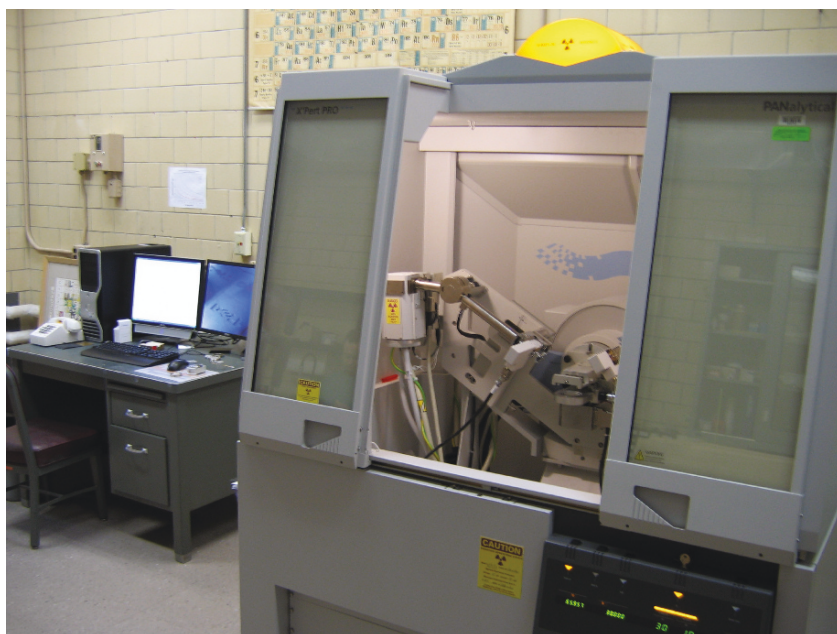
Fig. 11.4 The overall view of a powder diffractometer. On the right , the radiation enclosure is opened to expose the goniometer, which rests on top of the high voltage power supply. The computer on the left is used to manage and control data collection and to carry out preliminary processing of the data, e.g., conversion from a software-specific binary to ASCII format.
