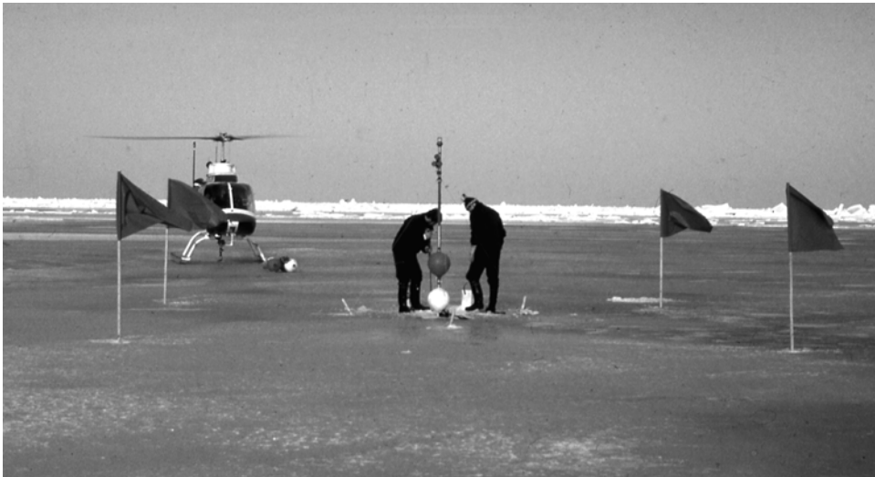
Figure 1.3. Deployment of a corner reflector mast for deformation studies by a laser geodimeter, in the Baltic Sea in April 1978. A system with several reflector sites allows accurate monitoring of sea ice kinematics in a 5 km scale array.
