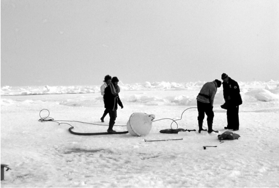
Figure 3.3. Deployment of an Argos buoy during the Ymer-80 expedition, July 1980, north of Svalbard. Argos buoys have provided fundamental knowledge about sea ice drift climatology in the polar oceans.
