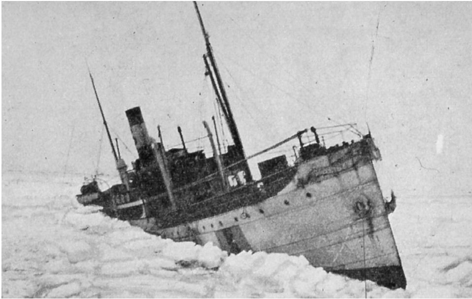
Figure 4.7. Ice pressure has captured one ship in the Baltic Sea. The strength of the ship is known but it is very difficult to predict local scale ice forcing from geophysical scale sea ice dynamics.
