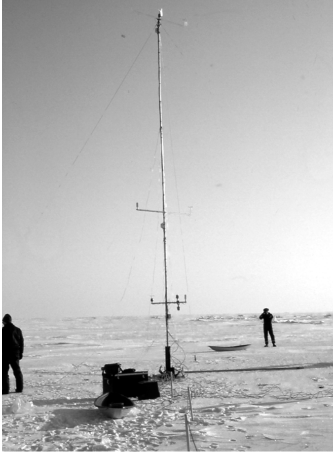
Figure 5.5. A mast (height 10m) for atmospheric surface layer measurements. Velocity, temperature, and humidity are measured at several altitudes to determine the fluxes using the so-called profile method.
