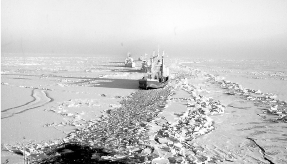
Figure 8.7. Convoy of ships assisted by an ice-breaker in the Baltic Sea. Ice dynamics determines the length of a convoy.
