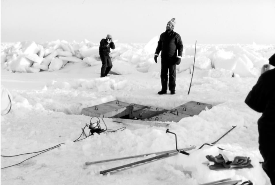
Figure 4.5. Field experiment into the strength of sea ice ridges in the Baltic Sea, winter 1987. The ridge keel is loaded by weights to examine the Mohr–Coulomb model.
