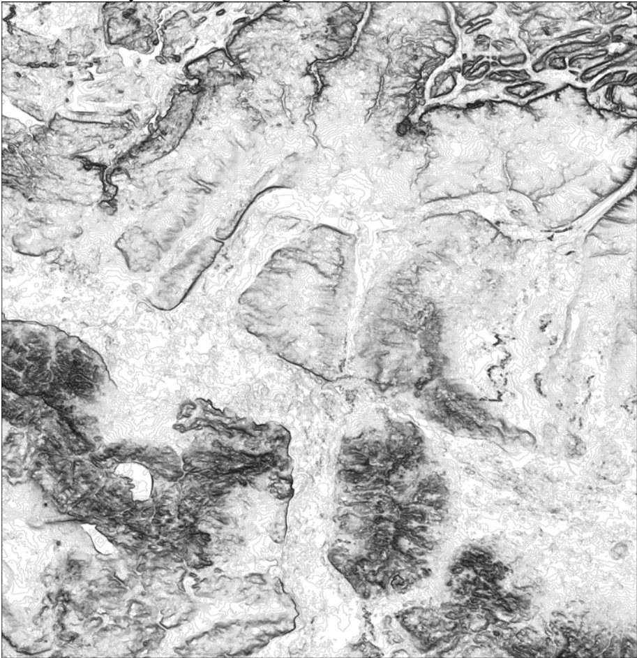
Figure 2. Condensed contourlines emphasize minute terrain features diffused or masked in the field by forest cover; DEM. Width of the picture is equal to about 70 km in terrain.
