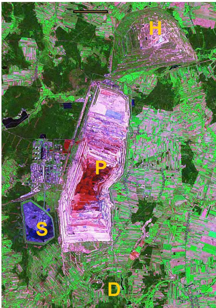
Figure 2. Landsat mosaics (NASA, courtesy MrSID); portion of the south central Poland; besides forests, meadows & arable lands, uncovered soil and subsoil, and settlements there are recognizable details of: H – spoil dump, P – open-pit lignite mine, S – settlement pond, D – dewatering screen surrounding the salt diapire; the upper bar is 2 km long.
