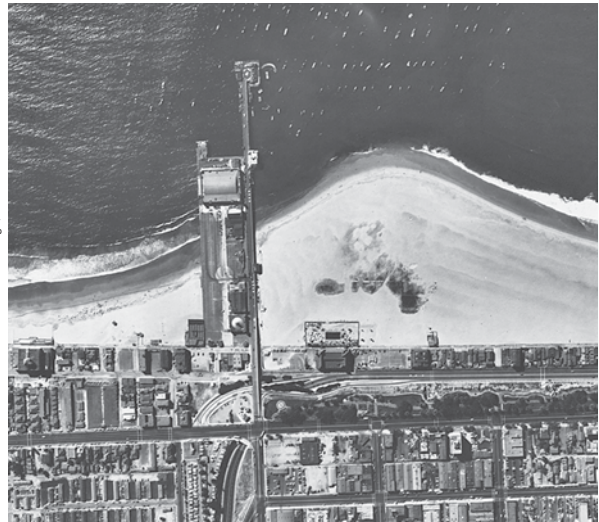
(b) The same shoreline in 1949 after the breakwater was built. The boat anchorage formed by the breakwater is filling with sand deposited by disruption of the longshore current.
