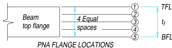
Fig. 5-3. Composite beam table parameters.
