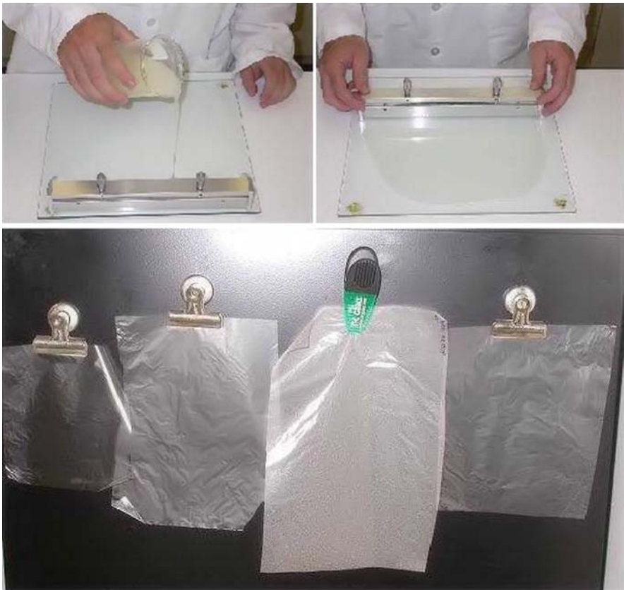
Fig. 3.2 A simple lab process for making gum films
