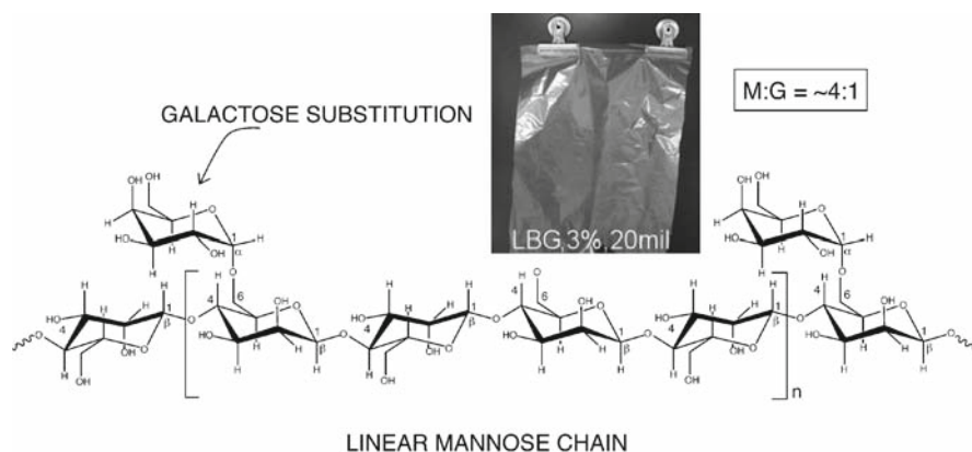
Fig. 3.20 Structure of locust bean gum and picture of its film, cast from a 3% solution and thickness of 20 mils (0.02 in. and 508 \mu m)
