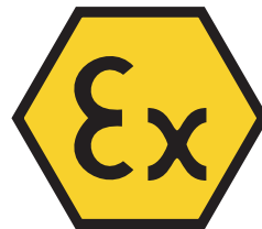
Fig. 65 Official symbol for marking equipment and protection systems intended for use in hazardous areas
