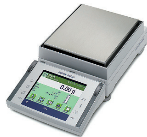
Fig. 135 Precision balance with a weighing capacity of 4 kg and a readability of 0.01 g
