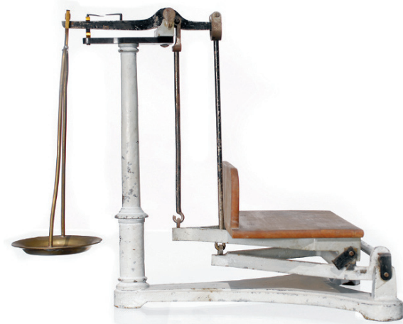
Fig. 38 Decimal balance (Image by courtesy of Pfunds Museum Kleinsassen/Rhön, Hofbieber-Kleinsassen, DE)
