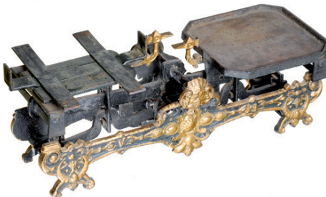
Fig. 19c Lever system of a Béranger flat-pan scale
