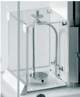
Fig. 97 Hanging (low-level) load receptor
