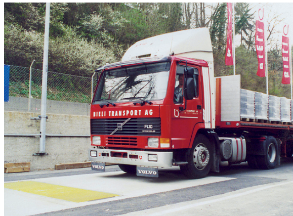
Fig. 51 Dynamic axle-load scale (Image by courtesy of Digisens AG, Murten, CH)
