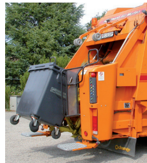
Fig. 75 Garbage truck with integrated scale (Image by courtesy of Digisens AG, Murten, CH)
