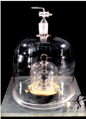
Fig. 88 Pt-Ir facsimile of the International Kilogram Prototype at the BIPM in Sèvres, Paris (Image by courtesy of BIPM, Sèvres, France)
