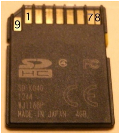
Figure 8-1. SD card pinout
