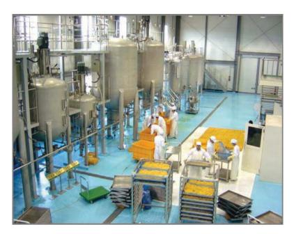
Fig. 12 Production of Panax ginseng adventitious roots in 10-ton scale bioreactors
