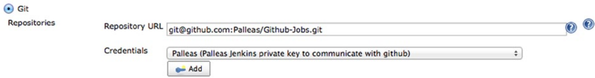
Figure 5-6. Explicitly selecting the credentials allows Jenkins to communicate with the Git repository
