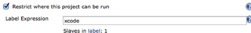
Figure 5-17. The application will be built on a slave that can run xcode
