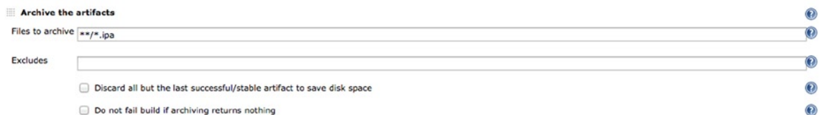
Figure 5-7. Asking Jenkins to find and archive the ipa files at the end of the build
