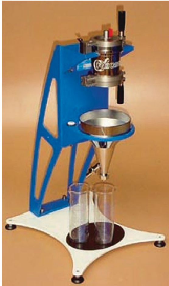
Fig. 3.5 Canadian Standard Freeness tester (Photo courtesy of Thwing-Albert Instrument Company)
