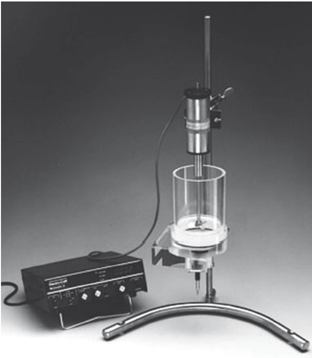
Fig. 3.6 Britt Dynamic Drainage Jar (Photo courtesy of Paper Research Materials Inc.)
