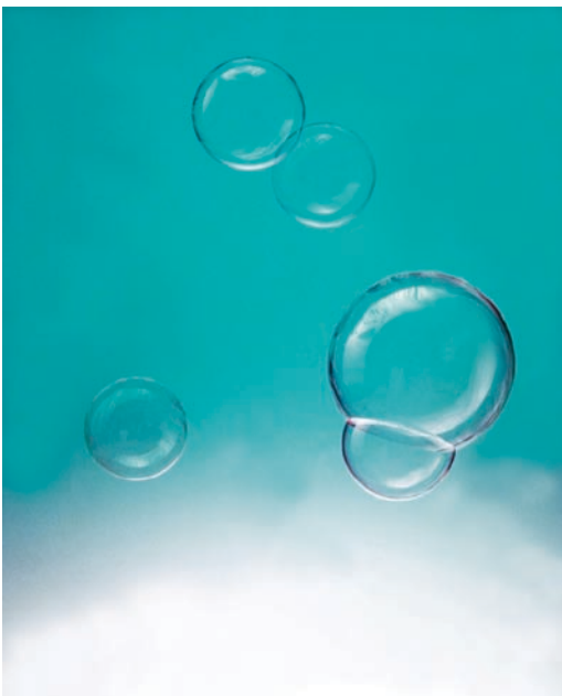
Fig. 4.7 Photograph showing bubble coalescence
