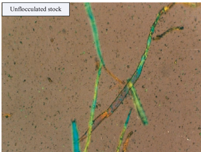
Fig. 3.1 Unflocculated stock – the fines and filler are apparent in the water phase
