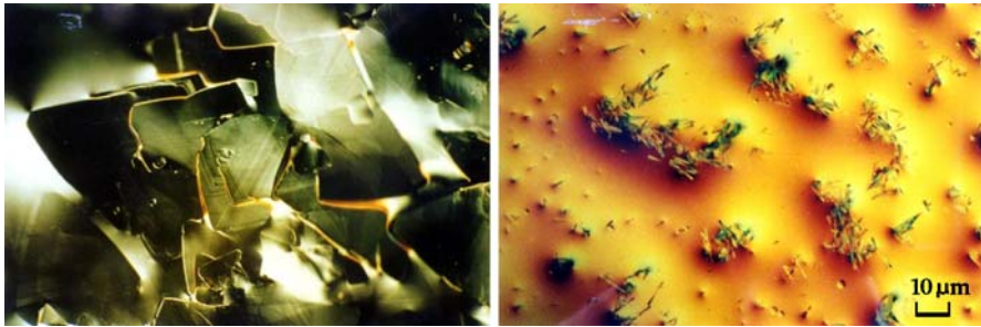
Fig. 25 Micrographs, at -13\text{ }^{\circ}\text{C} , of an untreated ( left side ) and treated ( right side ) diesel fuel
