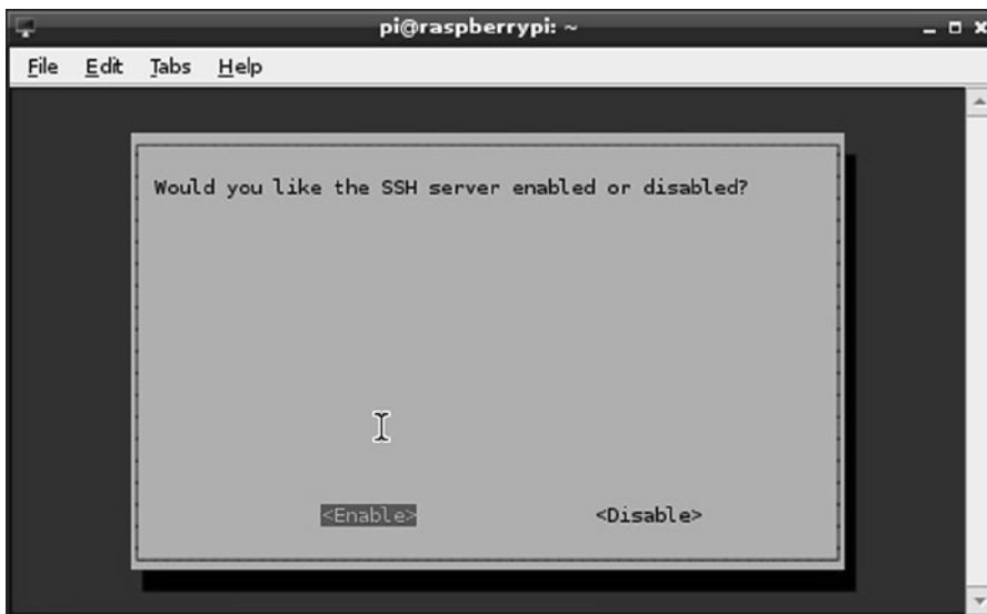
Figure 8-3. Enabling the SSH server
