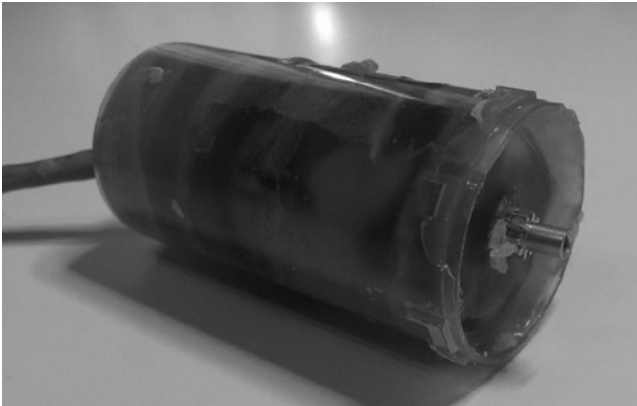
Figure 12-14. Motor surrounded by wax
