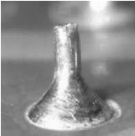
Figure 4-18. A good solder joint
