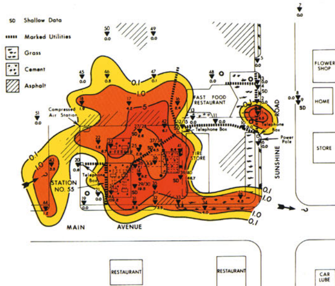
Fig. 5-65 Hexane ( C_5 ) concentrations (in ppm) in XYZ Gas Station. Seepage is occurring toward the top and right side of the map (reprinted with permission from Scientific Geochemical Services).
