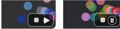
Figure 7-2. Custom button panel control having Stop (rectangle), Play (triangle), and Pause (circle) buttons
