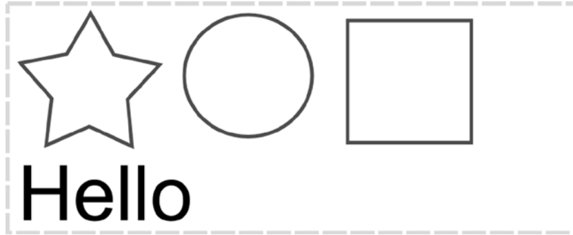
Figure 4-5. A FlowPane layout with nodes flowing left to right with the ability to wrap nodes based on horizontal space. The Hello text node is wrapped to the next line because the available horizontal space, denoted by the dashed line, is too small
