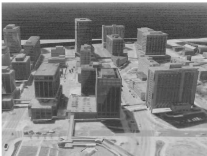
Figure 6-8. Digital elevation model of Rosslyn, Virginia derived using metric aerial photography and soft-copy photogrammetry software. The aerial photography is draped over the digital elevation model.
