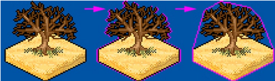
Figure 5-8. Hull generation process. Per scan-line, you find the min-max pixels for that row and toss those at a convex hull generator
