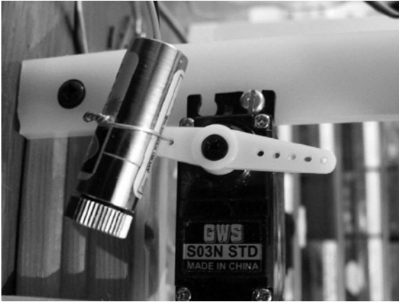
Figure 2-4. Laser diode mounted on servo motor
