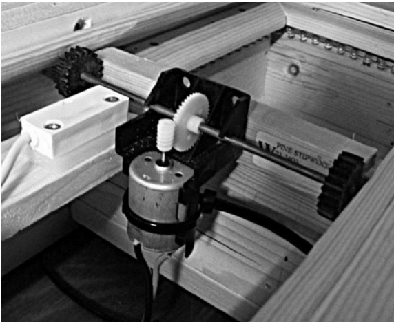
Figure 1-6. Panel drive assembly (with motor)
