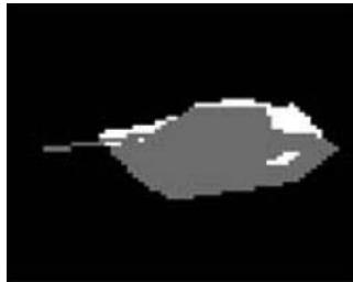
Figure 16.2. 2D encoded LADAR range image used as a training target.
