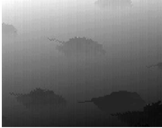
Figure 16.3. 2D encoded input LADAR range image with a training target at the right bottom corner.
