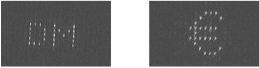
Figure 17.15. Diffraction patterns of the optical phase elements used for the demonstration experiment: (a) diffraction pattern of the integrated decryption key and the “real” kinegram TM and (b) diffraction pattern of the forged kinegram TM .
