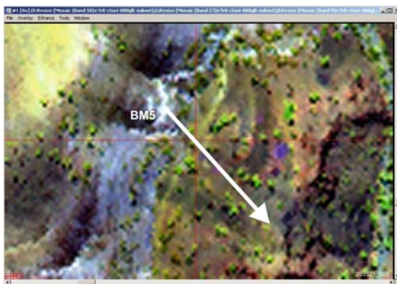
Fig. 5 HyMap imagery (1268,816,543:RGB) over Blue Mine showing the surface projected line of drill hole BM5
