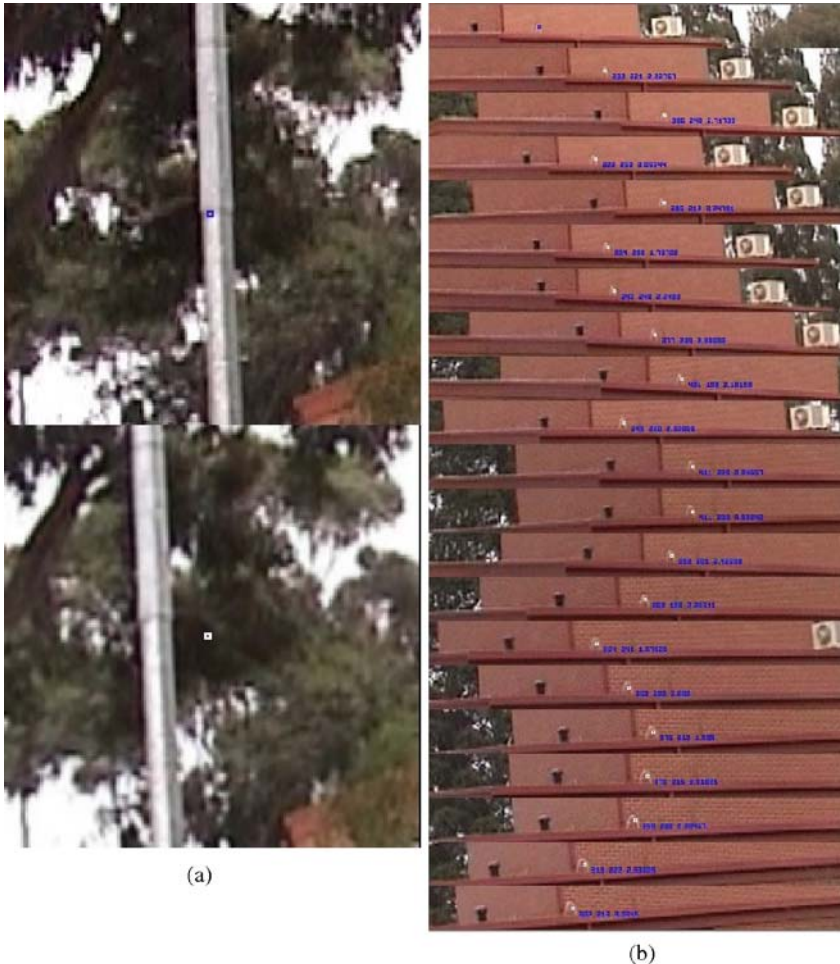
Fig. 5 (a) Using phase correlation for matching can sometimes give incorrect results. A crop of two consecutive frames with a point on the pole incorrectly matched to the position which was behind the pole in the previous frame. (b) A feature point tracked through multiple frames. Only the 20 pixels above and below the feature are shown from each frame.
