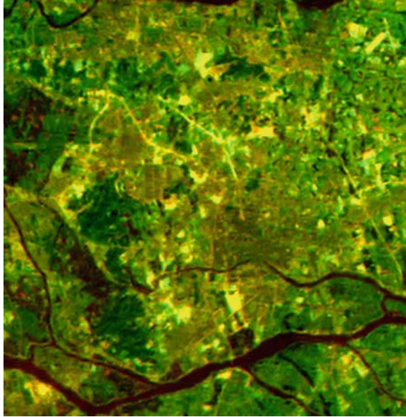
Fig. 7 Zoomed area on the composed image (CCD image Band 3 as the red channel and IRMSS band 2 as the green channel. IRMSS image pixel resolution was resampled from 75 into 25 m)
