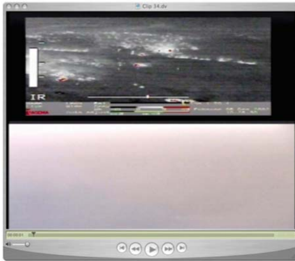
Fig. 6 This image taken 5 Dec 2002 near Borowra shows the difference FLIR can make to critical intelligence collection. (Top image is TIR and bottom image is the visual bands). Without FLIR the bottom view is all the crew can see
