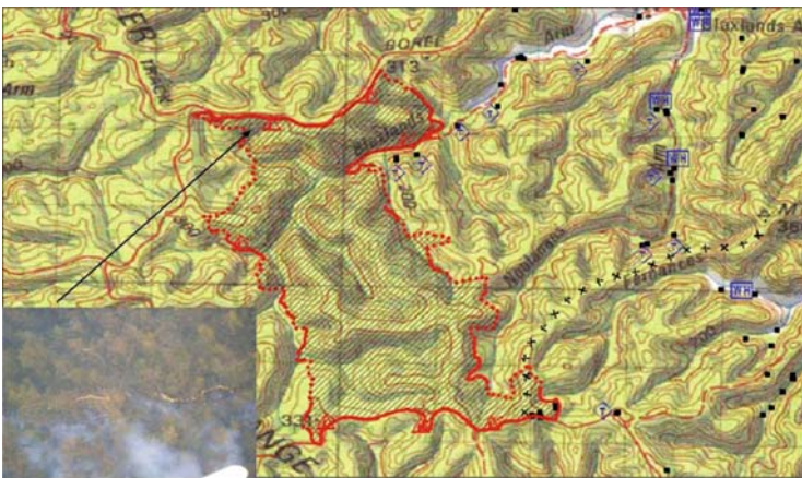
Fig. 4 Screen shot of a PyroMap fire plot that has a hot-linked digital hand-held camera photo (Bottom left) to indicate fire behaviour
