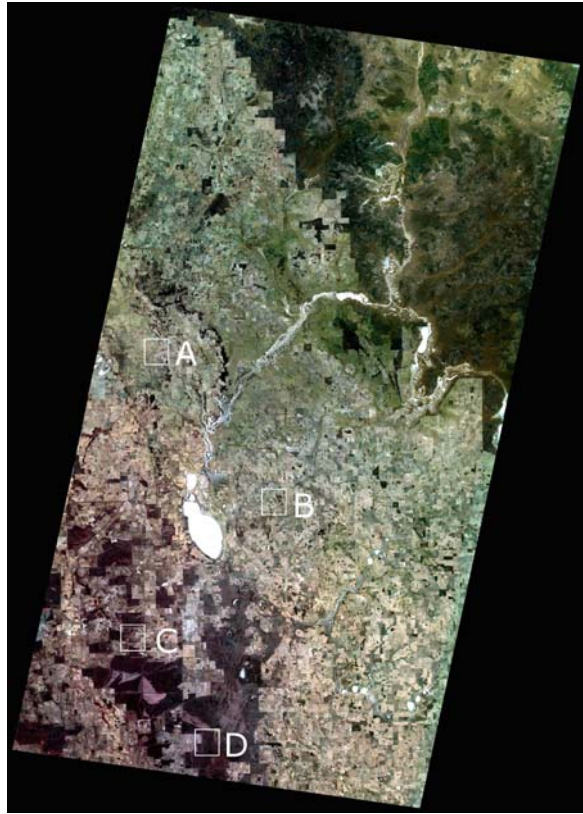
Fig. 5 CBERS WA dataset (combined two scenes of row 132 and row 133 at path 358), acquired on February 7, 2005, in the Land Monitor project region, Western Australia. The scene contains CCD bands 4, 3 and 2 (represented by red, green and blue colours, respectively)
