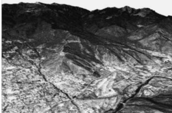
Fig. 3 Visualisation – orthorectified pansharpened image draped over DSM
