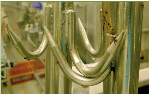
Surfaces that are in direct contact with meat must be made of stainless steel.
