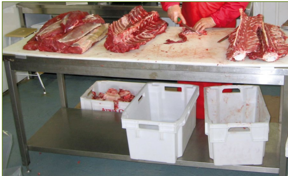
Industrial plastic cutting boards are suitable surface material for meat cutting tables.
