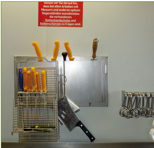
The utensils used for slaughtering must be easy to clean and disinfect and they must be stored appropriately (Photo: courtesy LEVO company, Lower Austria).
