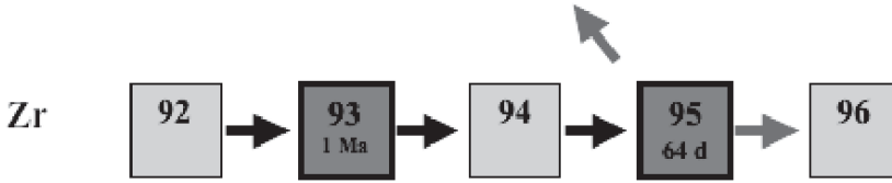
Figure 7: Small section of the chart of nuclides, showing the branching at ^{95}\text{Zr} . The s process proceeds by adding neutrons to both stable (light grey) and unstable (dark grey) species. Radioactive species like ^{95}\text{Zr} can either \beta -decay or capture a neutron.
