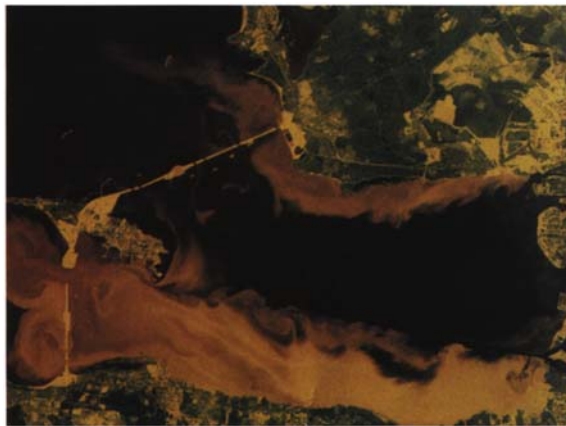
Plate 8b (Figure 5.88) The Neva Bay. Photograph taken from Soviet satellite on 5 July 1989. 10:36 Moscow time, height 278 km, original scale 1:200000. Colour film. The image shows large areas of a suspended matter field after construction of the Flood Barrier.
