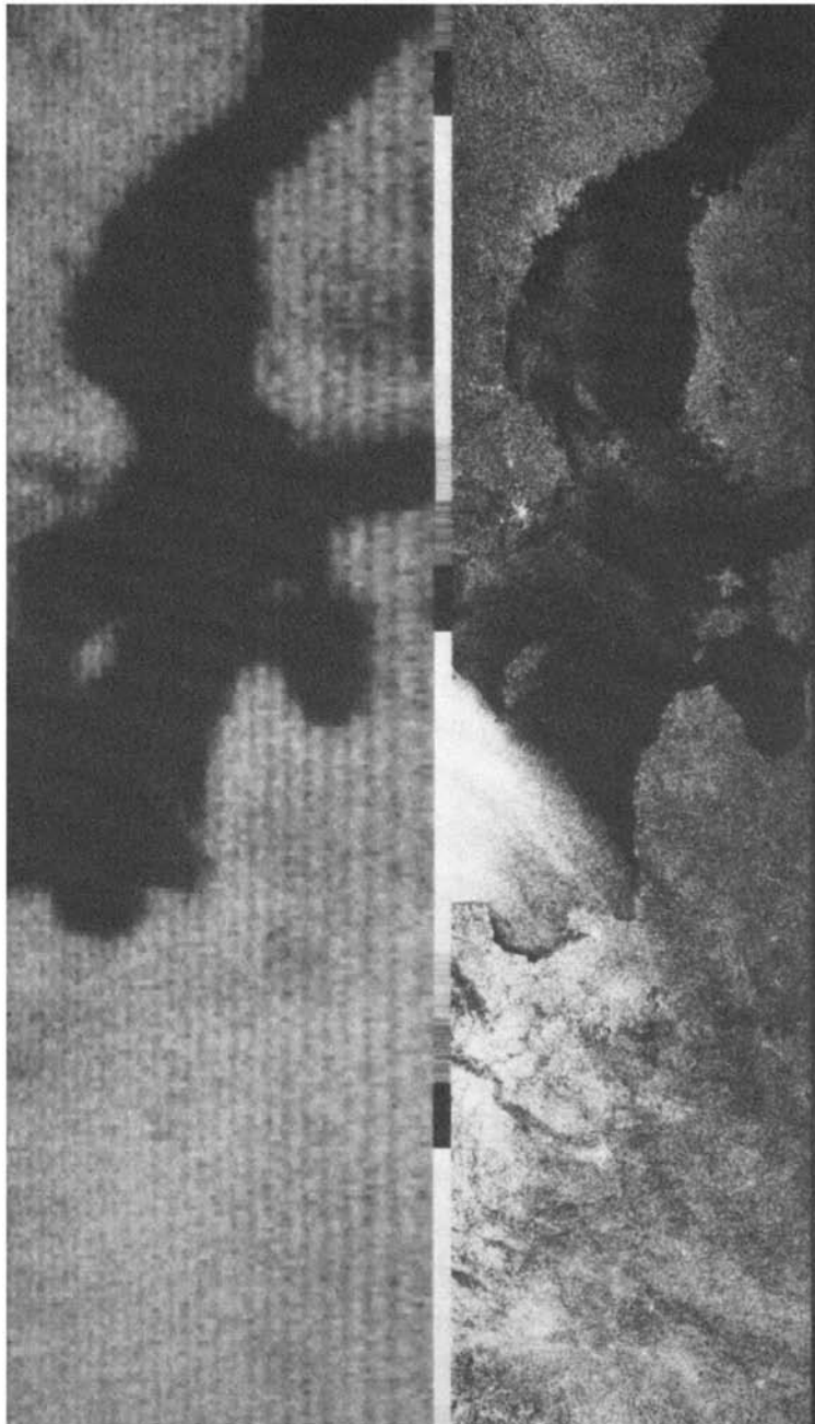
Figure 2.2 Full-resolution frame transmitted from the OKEAN-1 satellite on 3 September 1988 (main acquisition Centre/Moscow). A large part of the Baltic Sea is covered. The left part is the image from the microwave radiometer RM-08 (no useful information for regional satellite oceanography). The right part is the image from the side-looking radar. Sea surface roughness anomalies can be seen. The bright spots on the coast are the big cities of Stockholm, Riga and Turku.
