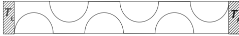
Figure 2. The geometry of the Lorentz gas channel model. The two heat reservoirs at temperatures T_L and T_R are indicated.
