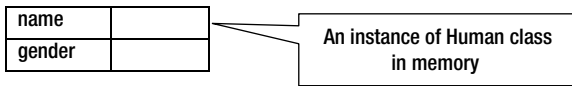
Figure 6-1. An instance of the Human class in memory created by the new Human() instance creation expression
