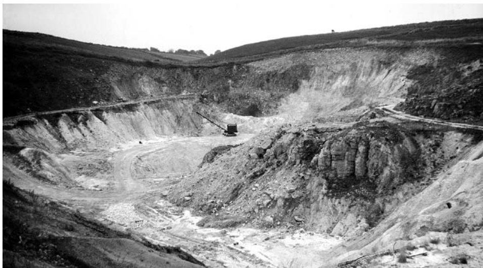
Figure 5.5. A large buried sinkhole in England's southern Pennines, exposed after its fill was extracted as a valuable source of refractory minerals; scale is indicated by the old excavator. TW.
