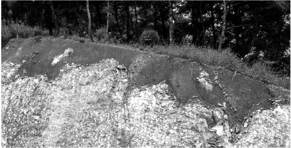
Figure 5.6. Two small limestone “floaters” within a red, clay-rich soil above a rockhead of only modest relief exposed in a new road cut in Korea. TW.
