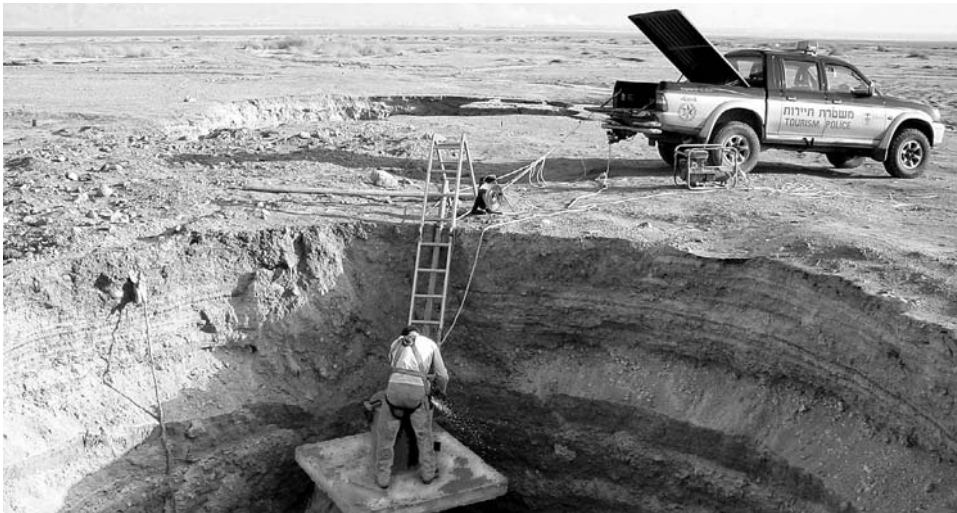
Figure 9.8. A man standing on the collar of a borehole that had dropped into a sinkhole over salt in the Israeli desert near the Dead Sea; though dissolution, cave development and sinkhole formation were already active in the area, the location of this sinkhole was determined by the borehole that was drilled to investigate the subsidence problem.
