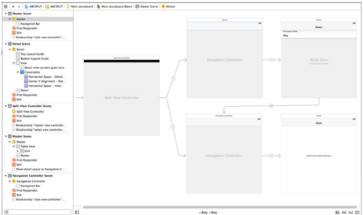
Figure 11-6. MainStoryboard.storyboard open in Interface Builder. This complex object hierarchy is best viewed in the Document Outline
