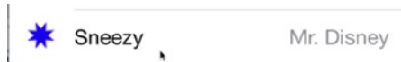
Figure 8-11. The style value 1 will place the text label on the left side in black letters and the detail text right-justified on the right side in blue letters
