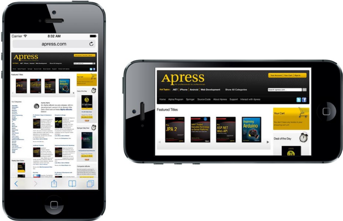
Figure 5-1. Like many iOS applications, Mobile Safari changes its display based on how it is held, making the most of the available screen space
