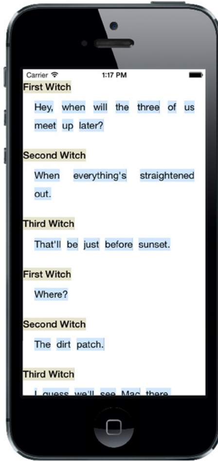
Figure 10-1. Each word is a separate cell, with the exception of the headers, which are, well, headers. All of this is laid out using a single UICollectionView , and no explicit geometry calculations of our own
