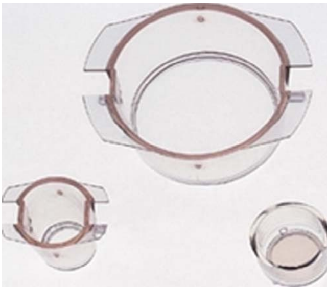
Figure 5.8 Culture inserts. The different models of culture inserts used for cultivation of limbal epithelial cells with feeder layers, acting as a barrier between the feeder layers and the growing limbal epithelial cells, and provide an air–liquid interface when the level of the culture medium is lowered.
